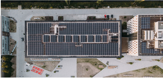
Fig. 4. Energy generation via 1,200 solar panels on the rooftop of the 'Echo', TU Delft (source: UNStudio/architectural record)
