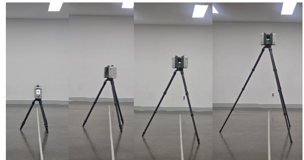
Fig. 3. LiDAR RTC 360 height setup (H1-H4)
