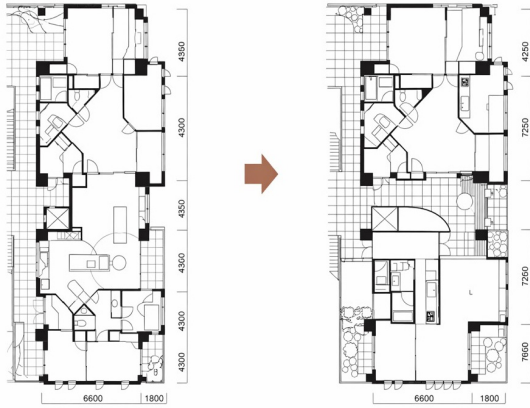
Fig. 1. Next21: Skeleton/infll-based flexibility and maintenance accessibility (shared-service management structure)—Reconstructed by the author based on public materials and presentation slides [12]
