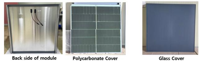
Fig. 2. Front and rear views of PV modules with colored glass or colored PC as the front material
