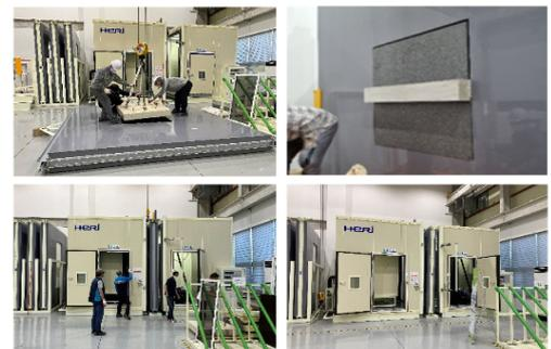
Fig. 5. Process of installing the wall-slab structural specimen
