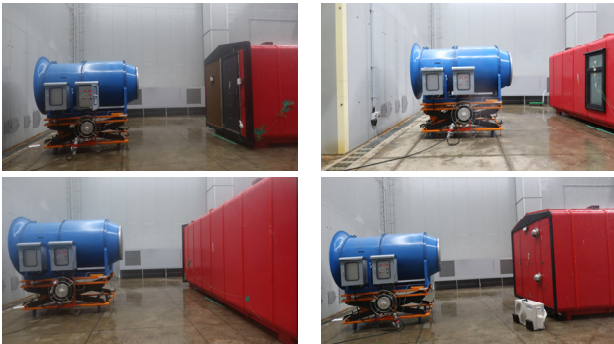
Fig. 8. Waterproof performance experimental procedure (Front, right, left, back in that order)
