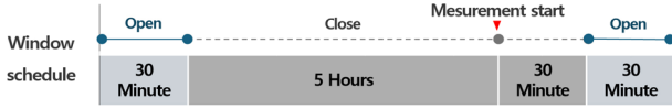
Fig. 10. Measurement of indoor air quality in residential building B1, B2, B3 - window opening/closing schedule
