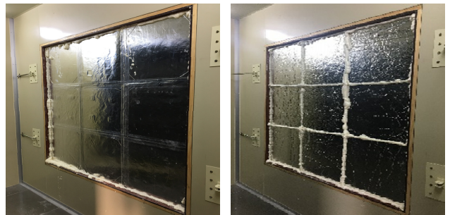
Fig. 8. Thermal transmittance test facility
