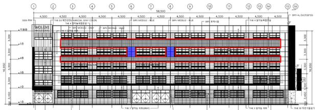
Fig. 9. Design and area of BIPV in the facade of the south of middle school
