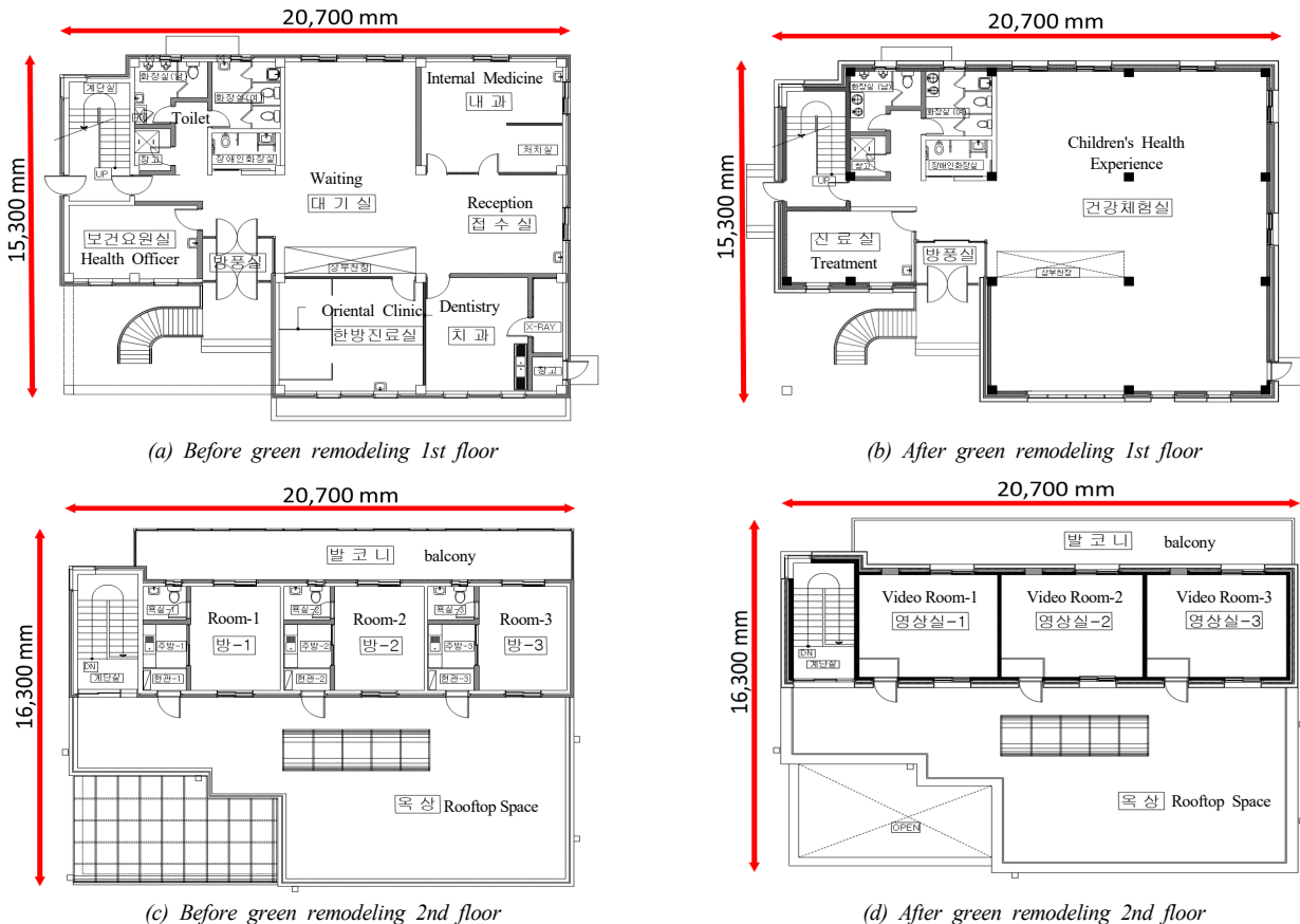
Fig. 5. Floor plans before and after green remodeling
