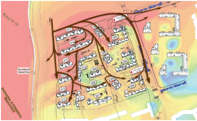
Fig. 23. Particulate Matter movement path after 75 minutes
