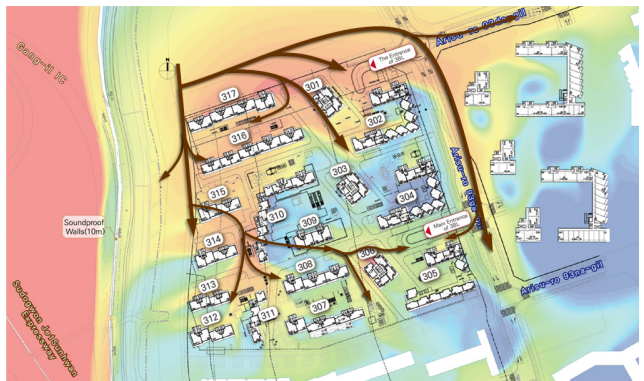
Fig. 19. Particulate Matter movement path after 45 minutes
