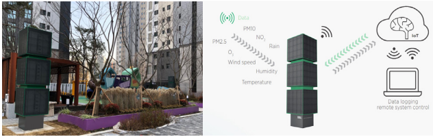
Fig. 4. Smart Filter Monitoring Cube (Source: mann+hummel)
