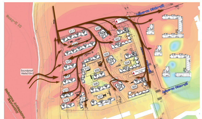
Fig. 25. Particulate Matter movement path after 90 minutes
