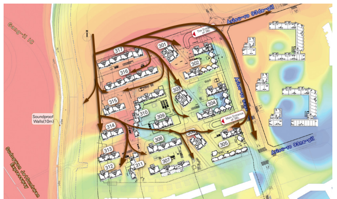
Fig. 21. Particulate Matter movement path after 60 minutes
