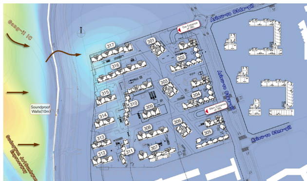
Fig. 15. Particulate Matter movement path after initial 15 minutes
