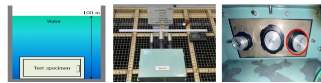
Fig. 13. IP X7 Specimen installation and result
