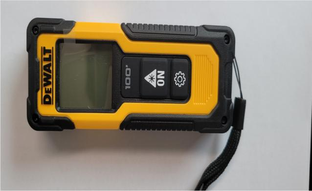
Fig. 5. Instruments used for field survey (DeWALT DWHT77100)
