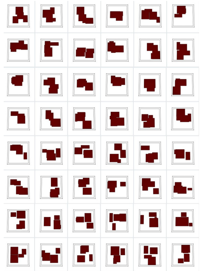
Fig. 8. Comprehensive design output (appropriate for building coverage ratio and high aspect ratio with a large number of south-facing locations)
