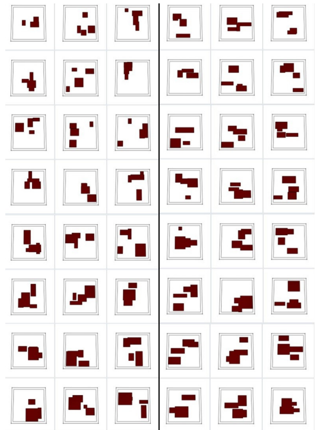
Fig. 5. Design output according to the difference in aspect ratio of the building (left: low, right: high)
