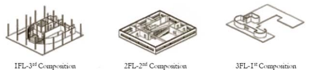
Fig. 14. Construction Process of Villa Savoye
