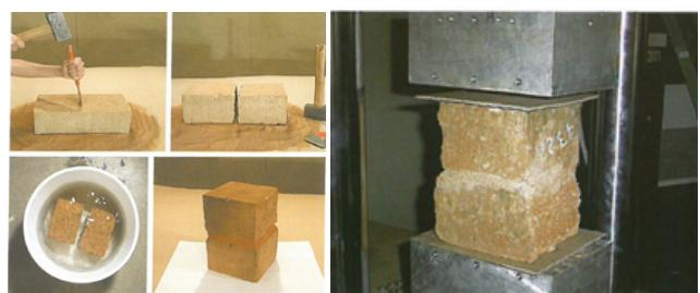
Fig. 8. Wet compressive strength test for earth block
