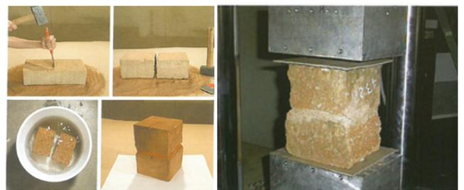
Fig. 8. Wet compressive strength test for earth block
