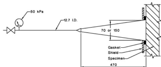
Fig. 11. Accelerated erosion test
