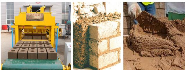
Fig. 2. Compressed earth block Fig. 3. Insulated earth masonry Fig. 4. Earth mortar
