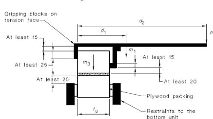
Fig. 9. Flexural tensile strength tests
