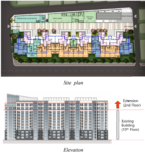
Fig. 2. Site plan and elevation of housing complex (After remodeling)
