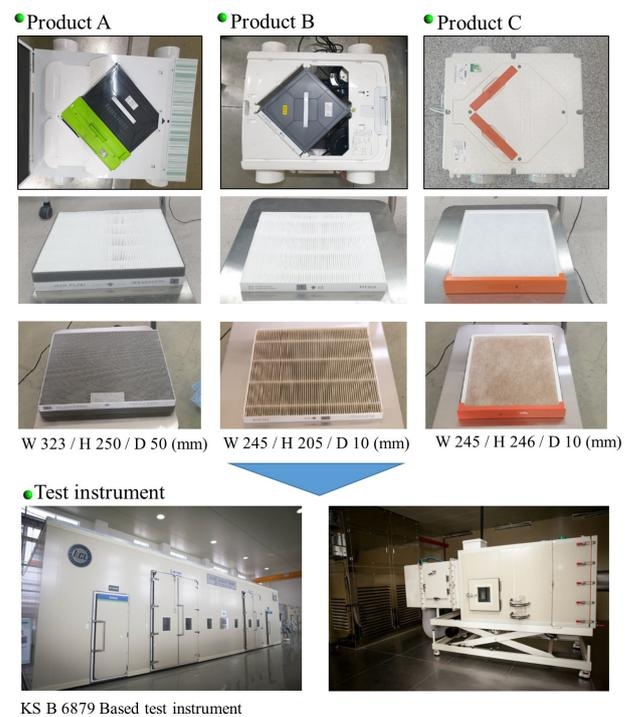
Fig. 4. Test sample of heat-recovery ventilators
