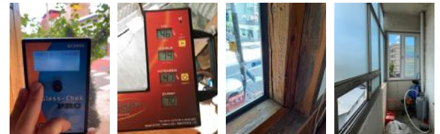
Fig. 2. Performance measurement and a field survey of window system
