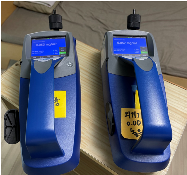
Fig. 6. Comparing of measurement differences between 2 TSI 8532
