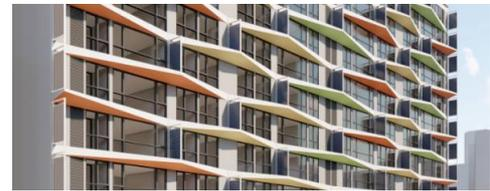
Fig. 3. LIPV (Louver Integrated Photovoltaic)
