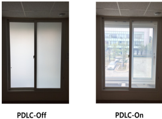
Fig. 12. Mock-up for Field Test of PDLC
