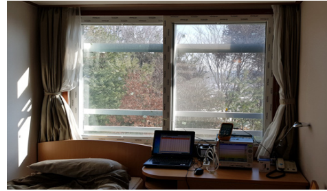
Fig. 9. Mock-up for Field Test of Heatable glass
