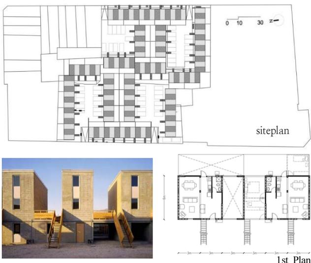
Fig. 1. site plan, first floor plan of Quinta Monroy
