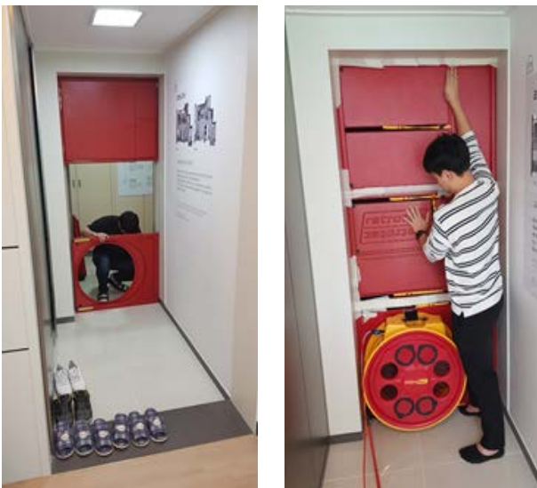
Fig. 3. Pictures for measurement using Retrotec blower door
