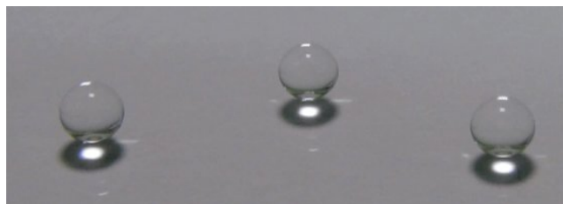
Fig. 3. Water on the Surface with Water-repellent Nano Coating [Source:CEKO]
