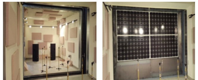
Fig. 13. Sound transmission loss test
