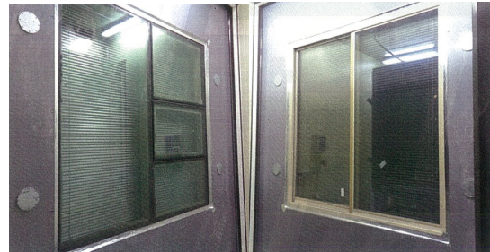
(a)cold chamber part (b) warm chamber part Fig. 3. U-value test according to KS F 2278
