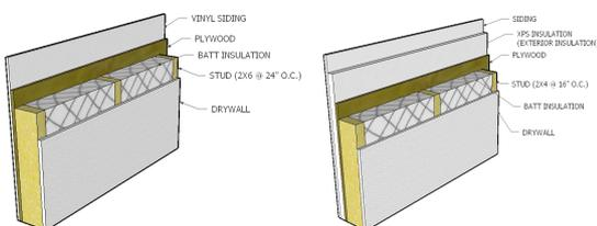
Figure 2. Wood frame wall with R-20 insulation (left) and R-13+5 insulation (right) as specified in the IECC 2015
