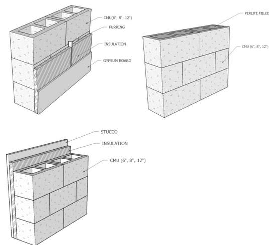
Figure 3. Three CMU wall insulation strategies: interior (top, left), integral (top, right), and exterior (bottom).
