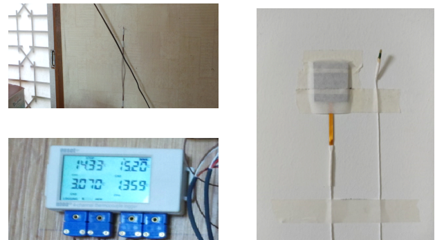
Fig. 3. In-situ measurement experiment(ASTR & HFM method)
