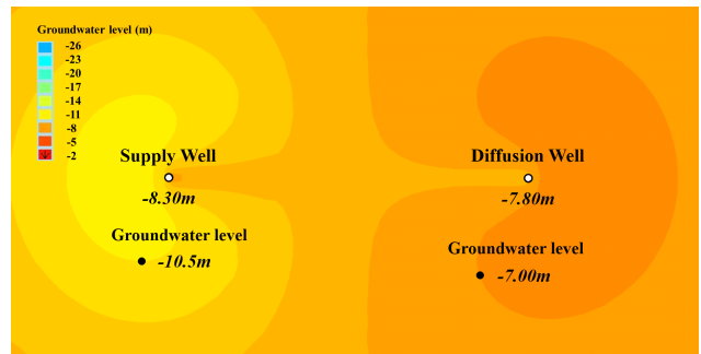
Fig. 7. Groundwater level of wells (Case 2-2, k:5 \times 10^{-7} \text{ m/s} , 2/28)
