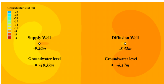
Fig. 4. Groundwater level of wells (Case 1-2, k:5 \times 10^{-7} \text{ m/s} , 2/28)
