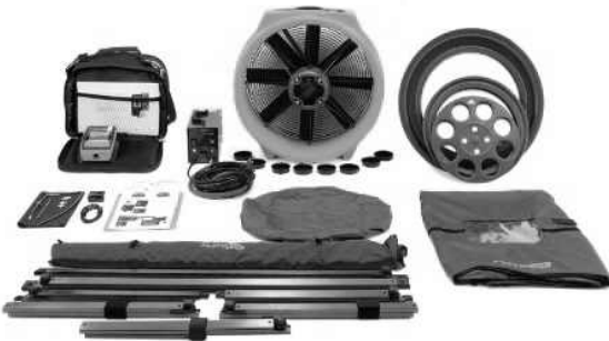
Fig. 2. Components of blower door
