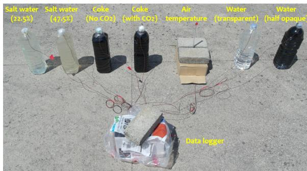
Fig. 6. A setting of temperature measurement to assess the performance of heat collection
