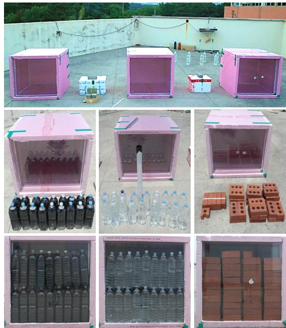
Fig. 9. Preparation of the three identical test cells (top) and materials (middle), and installation (bottom) for performance measurement
