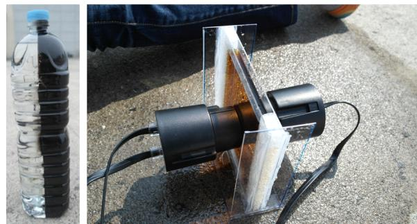
Fig. 5. A picture of half opaque water bottle (left) and measurement of visual transmittance (right)
