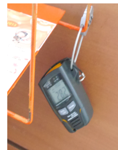
Fig. 7 Measurement of indoor temperature and humidity(B)
