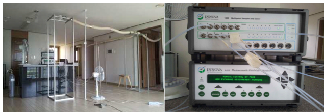
Fig. 4. Measurement of Ventilation Rate
