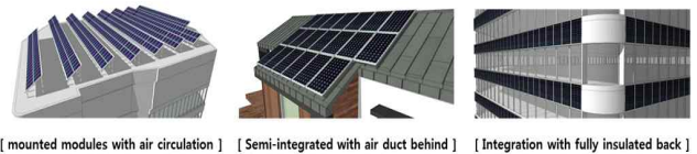
Fig 3. Installation types of PV systems
