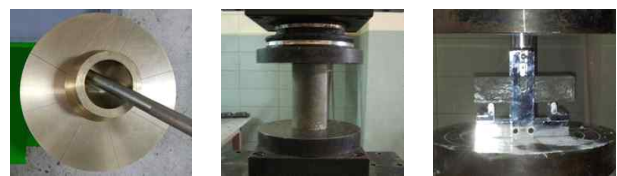
a) Slump flow test b) Compressive strength c) Flexural strength Figure 1. Test Methods
