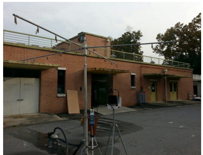
Fig. 2. Mist supply system
