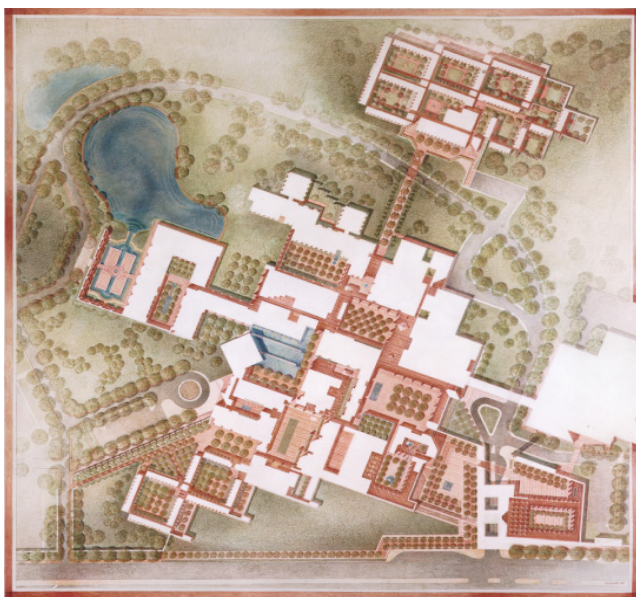
Fig.4. shows site plan showing west word orientation at macro level. With clear definition of courtyard type planning.
