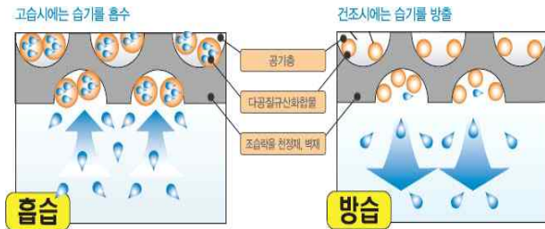
Fig. 1. Schematic diagram for moisture absorption characteristics
