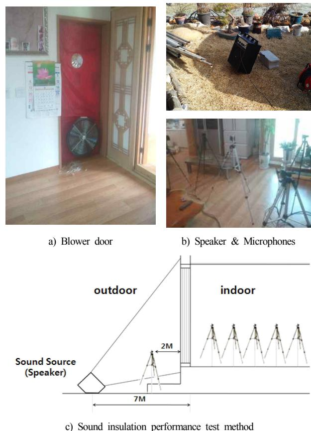
Fig. 1. Field measurement of Airtightness and Sound insulation performance
