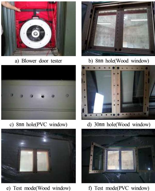
Fig 4. Opening types and test mode
