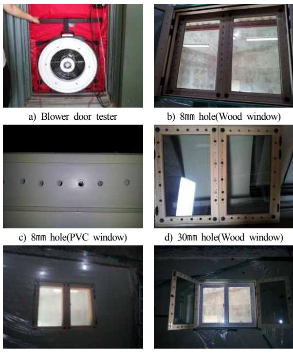
Fig 4. Opening types and test mode
